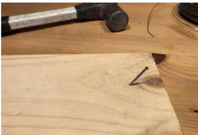
2. Loop the wire around the nail by tying a bowline, or loop-and-twisting, etc. Use pliers if needed. (Tuneable version: fully extend the turnbuckle, hook the eye on the nail, and fasten the wire to its other end.)
